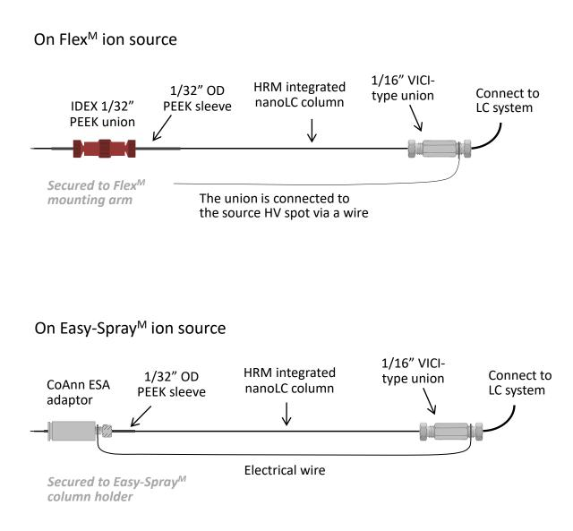
Note: Connection of the integrated column inlet and a nanoLC system can be done by using a CoAnn VHPCLD or a Thermo two-ends nanoViper.
