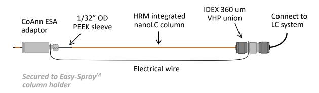
Note: the column connections can resist pressures up to 15,000 psi supported by the IDEX 360 um VHP union. A CoAnn VHPCLS or a Thermo one-end nanoViper can be used to connect column to a nanoLC system.
