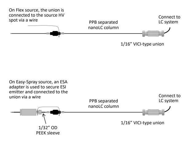
Note: Connection of the separated column inlet and a nanoLC system can be done by using a CoAnn VHPCLD or a Thermo two-ends nanoViper.
