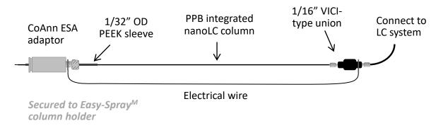
Note: Connection of the integrated column inlet and a nanoLC system can be done by using a CoAnn VHPCLS or a Thermo one-end nanoViper. The system can resist pressures of up to 8,000 psi.
