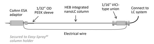
Note: Connection of the integrated column inlet and a nanoLC system can be done by using a CoAnn VHPCLD or a Thermo two-ends nanoViper.
