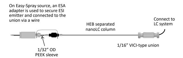
Note: Connection of the separated column inlet and a nanoLC system can be done by using a CoAnn VHPCLD or a Thermo two-ends nanoViper.
