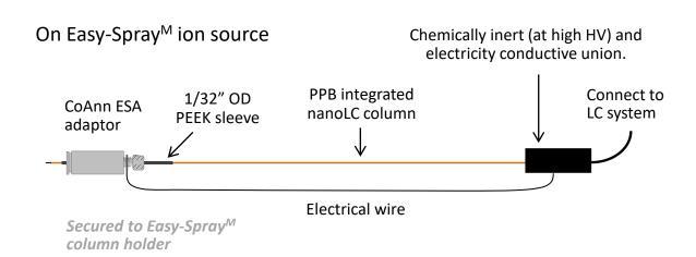
Installation of fitted CoAnn PPB integrated column on Thermo Flex<sup>M</sup> and Easy-Spray<sup>M</sup> ion sources
